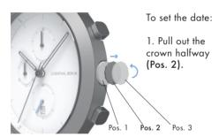
Turn the crown counterclockwise until the correct date is displayed.
