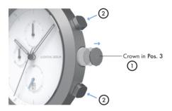
Pull out the crown to position 3 (1). Then press Pusher A and Pusher B SIMULTANEOUSLY for at least 2 seconds (2). The hands are now in reset mode.
